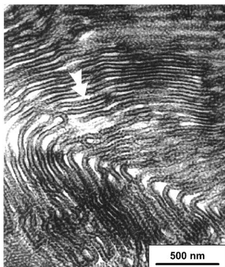
Fig. 10. Transmission electron micrograph of S_{35}B_{15}C_{50} .
